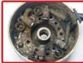
Although the outside of the starter (at bottom right) looks fine, the flywheel picked up water from the bilge and pumped it inside the starter causing the corrosion shown here.
