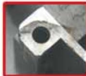
Shown here are damaged starter mounting pads. Water ingested into the engine stresses the mounting bolts beyond normal conditions. The bolts stretch and cause the starter to become loose. This could eventually lead to damage to the ring gear, starter casting and possibly the entire engine block.
