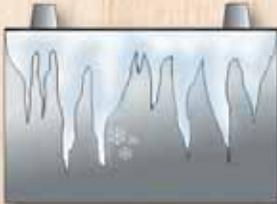
As a battery becomes discharged the percentage of sulfuric acid in the electrolyte becomes less. The sulfuric acid combines with the lead plates producing lead sulfate. As this happens **the electrolyte solution becomes pure water.** A discharged battery will freeze in cold climates, which will destroy the insulators and plates inside it.
