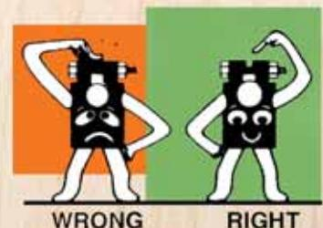
Make sure there is a gap between the ends of the terminal when tight.
