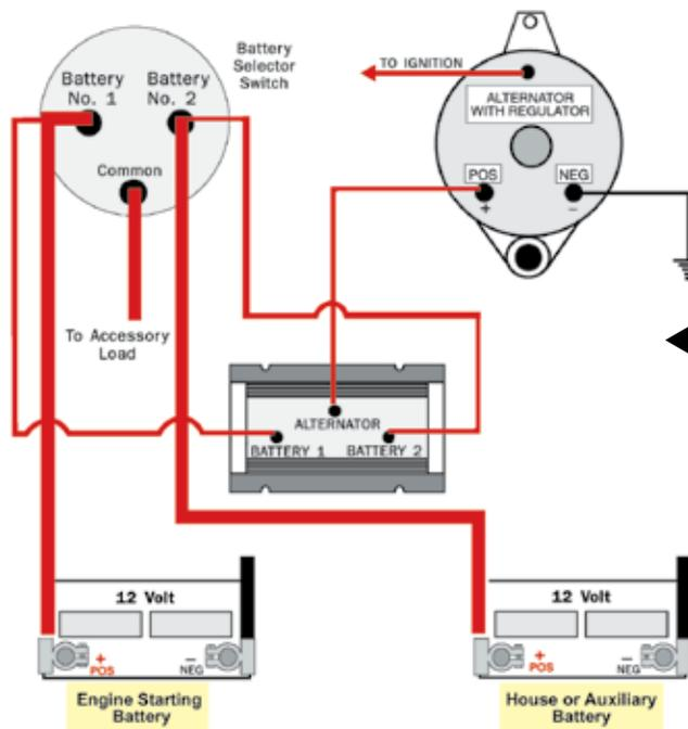
The two alternator, two battery isolator allows both alternators to charge both batteries.
