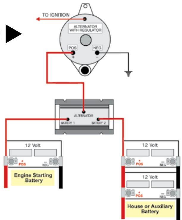
The one alternator, two battery isolator with a battery selector switch will allow both banks of batteries to be charged regardless of what position the battery selector switch is in.
