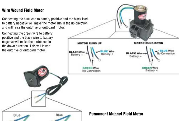
Connecting the blue lead to battery positive and the green lead to battery negative will make the motor run in the up direction. This will raise the outdrive or outboard motor.
