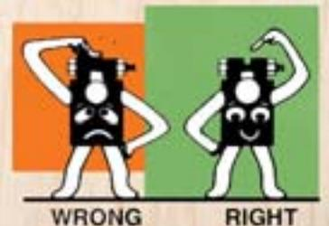
Make sure there is a gap between the ends of the terminal when tight.
